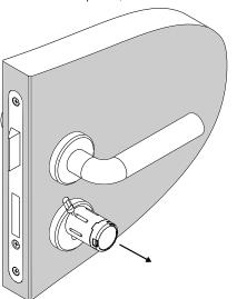
Remove the used battery and insert the new battery, paying attention to the polarity.
