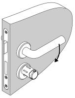
The time duration for which the knob cylinder remains engaged can be configured (1 to 15 seconds, the default value is 5 seconds). After successful authorization (engaging) at the knob, the engagement time countdown starts.
