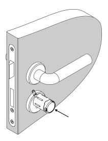
Check the time of the knob cylinder using the service unit CX6510 or ClexTouch CX6522 and adjust if necessary.
