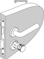
The knob module is now engaged and the door can be locked and unlocked by turning the electronic knob module.
