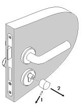
Remove the fixing screw.
