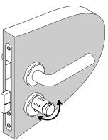
▶ The door can be opened using the door handle in the unlocked state.
