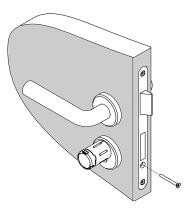
Remove the cylinder body and electronic knob from the lock.
