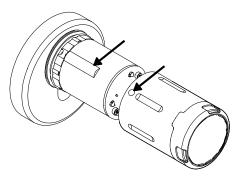
The knob cover has to be inserted such that only the rubber seal is visible. If this is not the case, hold the knob and turn the knob cover back and forth till the knob cover can be inserted up to the rubber ring.
